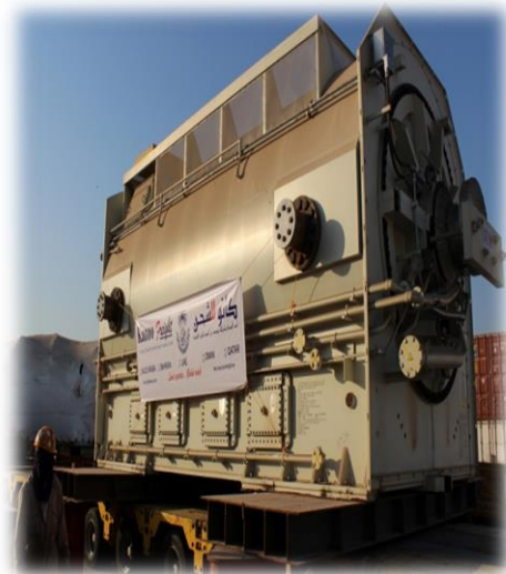
230 Ton Generator for Arabian Bemco PP12 Project from Dammam port to Dhurma Site Total 7 Units
